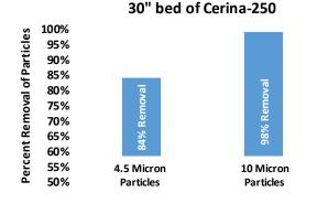
Filter Flow Rate 10 gpm/ft<sup>2</sup>
